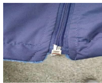
Photo 30) Major: Uneven edge at bottom
