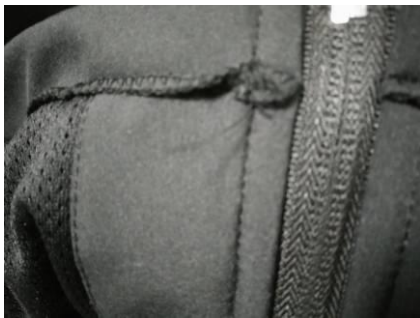
Photo 34) Minor: Untrimmed thread end at bottom
