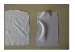
Photo 1) Two pieces test samples(left is dry fabric and right had been soaked in the soapy water)
