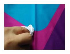
Photo 4) Color fastness test for wet Rubbing
