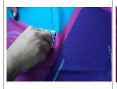
Photo 2) Color fastness test for dry Rubbing
