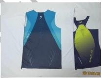
Photo 6) Color migration test(The color panel was sewn with white fabric at Sep 02,2015)
